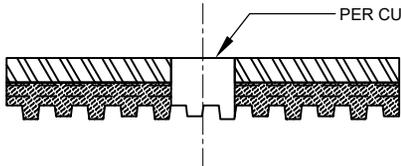
STYLE B - RIBBED WITH LOAD PLATE AND HOLE
