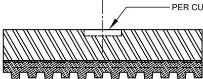
STYLE C - RIBBED WITH LOAD PLATE AND COUNTER-BORED HOLE
