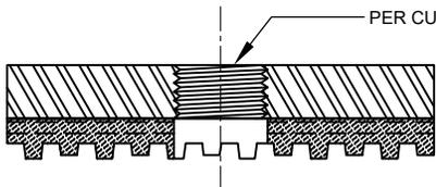
STYLE D - RIBBED WITH LOAD PLATE AND TAPPED HOLE
